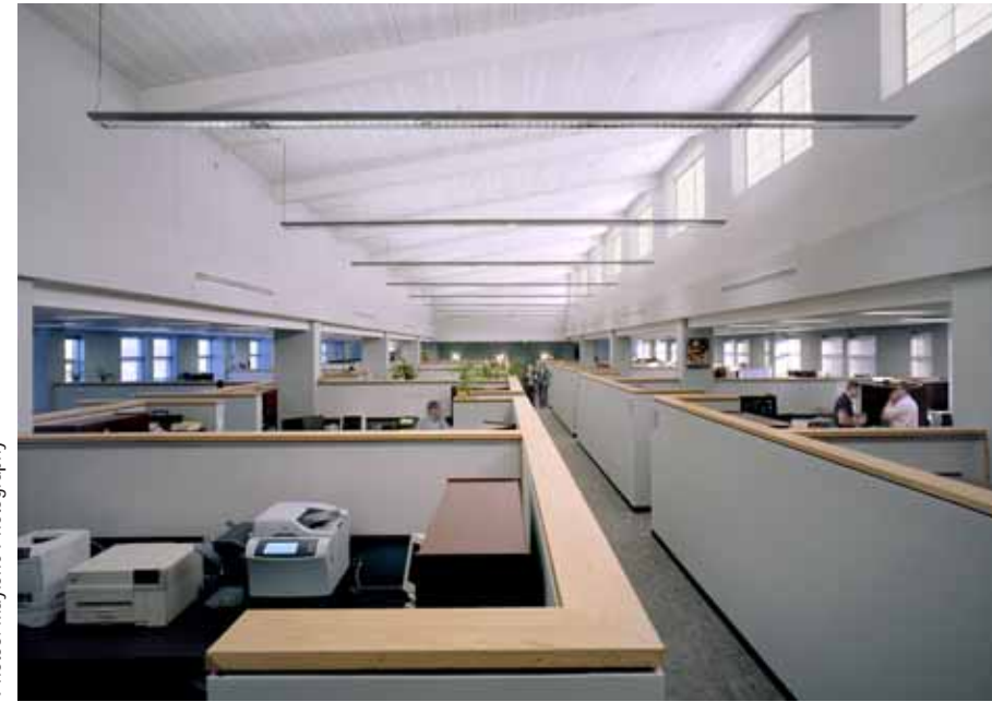
Interior light shelves and exterior sunshade louvers provide diffuse natural light in open-office spaces (above) and individual offices (right).
